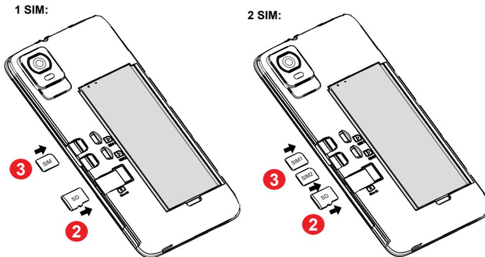
You must insert your SIM card to make phone calls. You do not need to power off your phone before inserting or removing the SIM card as this phone supports hot swap.
